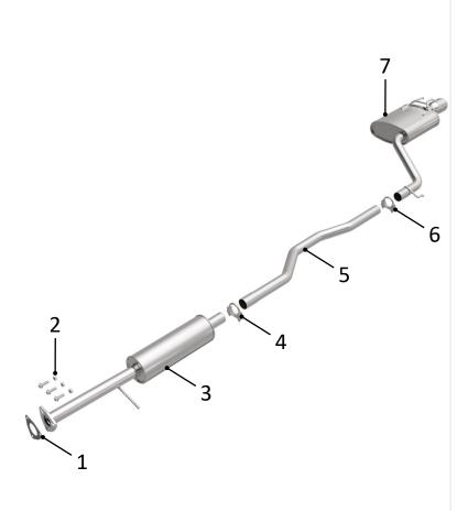
**STEP 1:** (Carefully read all instructions before installation) Disconnect the vehicle's battery before removal of the OEM exhaust system. This will prevent electrical accidents and will reset the computer if it applies to the vehicle. Remove existing exhaust system from the vehicle. Only remove parts that will be replaced. Clean existing flange with a wire brush to ensure proper sealing.
